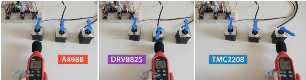
**Stepper driver noise levels:** A4988 around 65dB, DRV8825 around 67dB and TMC2208 around 41dB.
