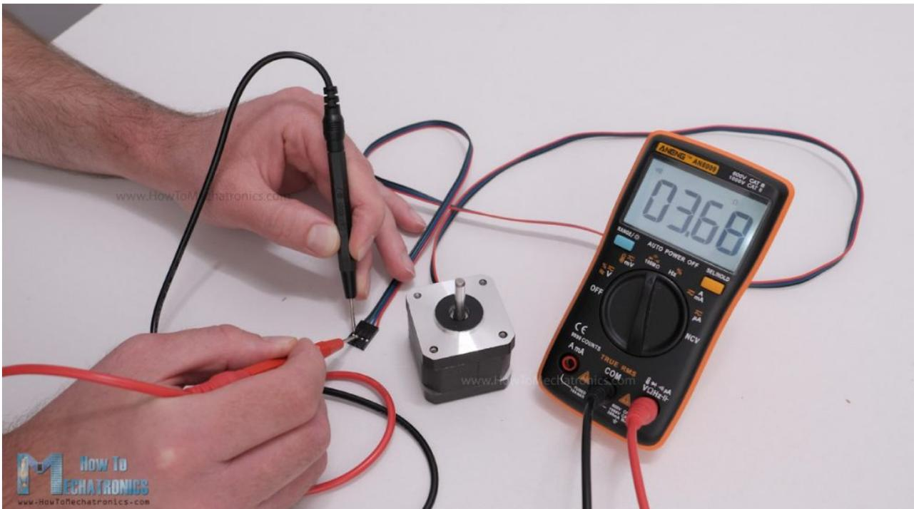
Once we find a phase, we can connect it to any position of the two positions on the driver, the order doesn't matter.
